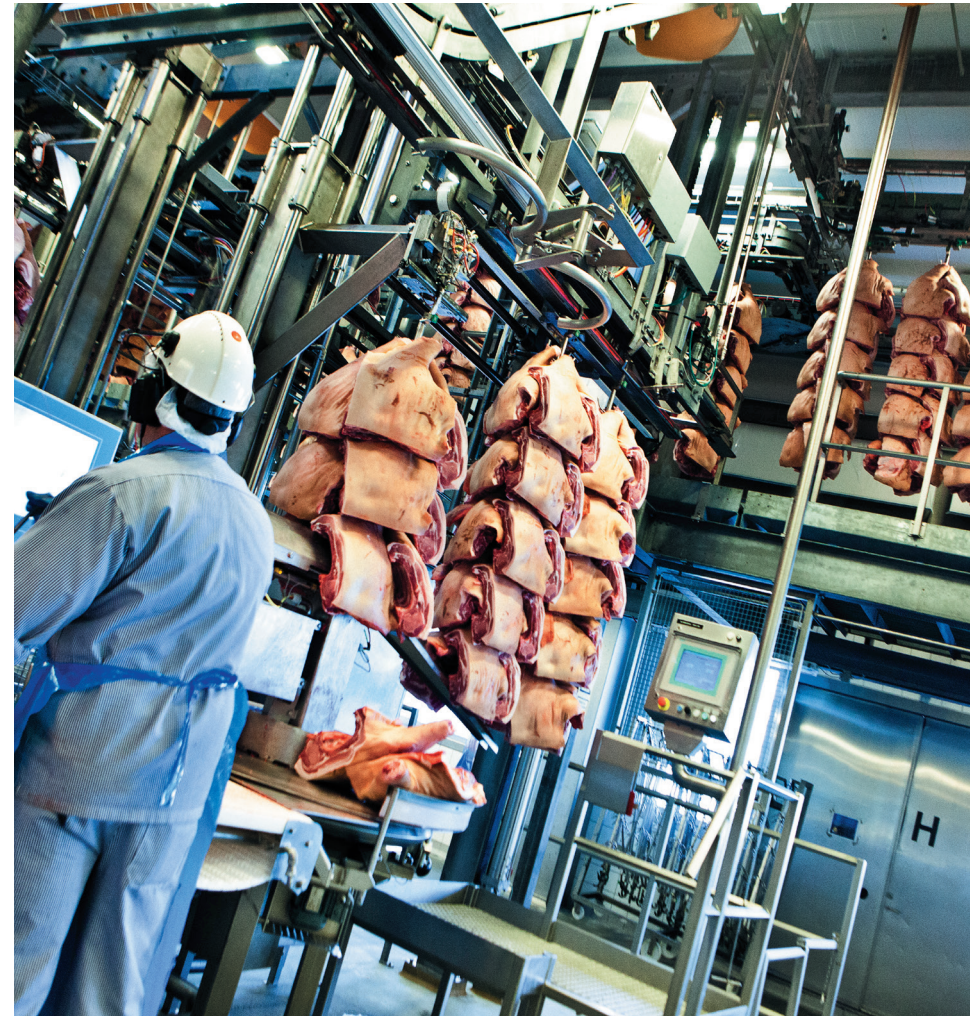
Frontmtec automatic transport of primal cuts hanging on christmas trees with RFID tags for traceability. Automatic and ergonomic unloading of primals, a task that is particular strainful when done manually.
