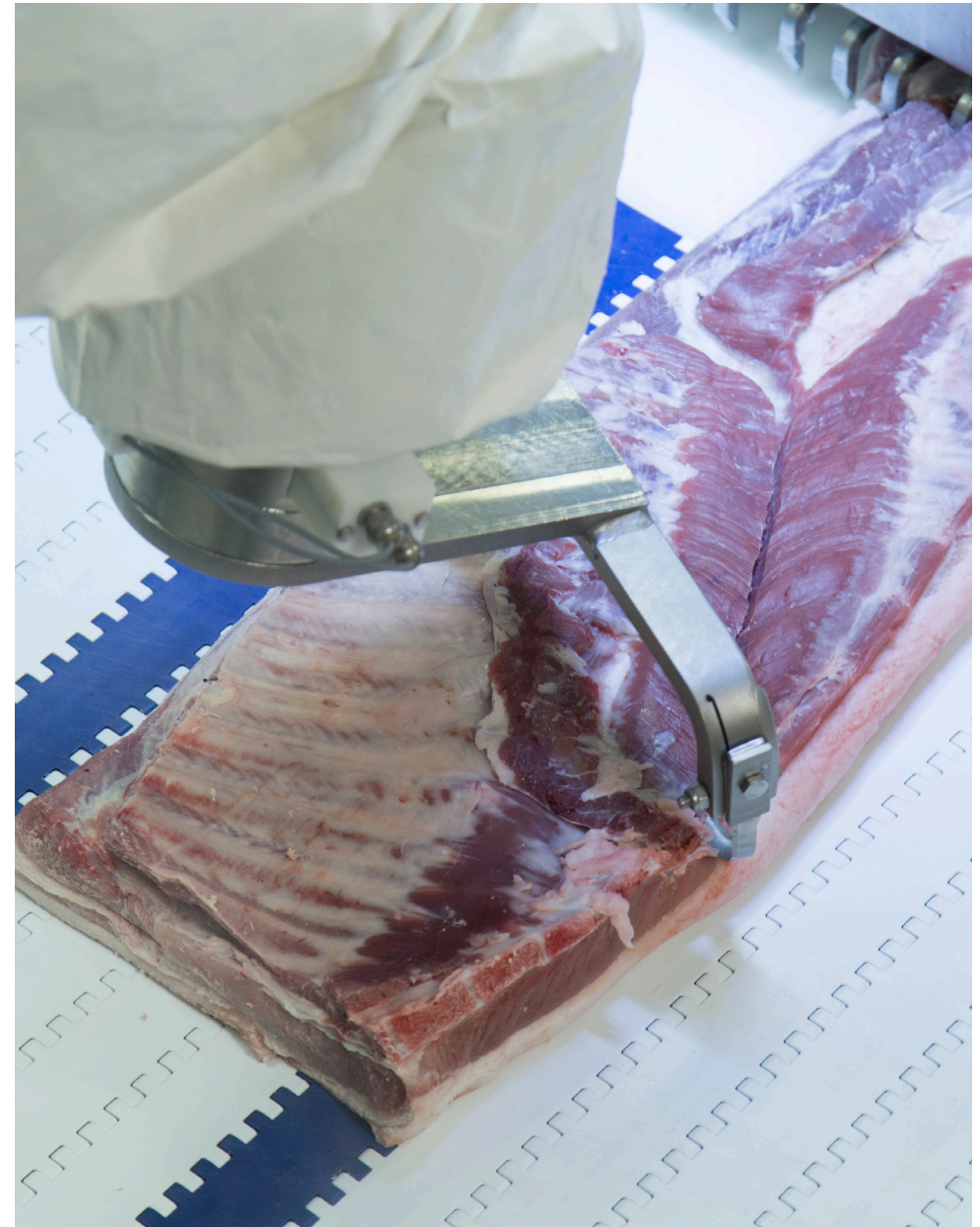
Frontmatec Automatic Rib Puller in operation. Replaces the manual physical demanding task of pulling ribs with a robot for improved yield.
